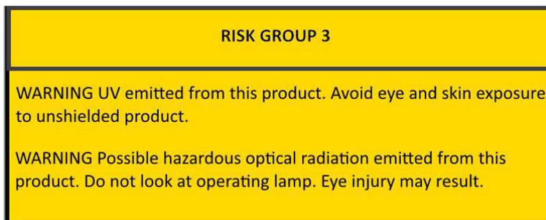
This label is attached to the reverse panel of the light source.
