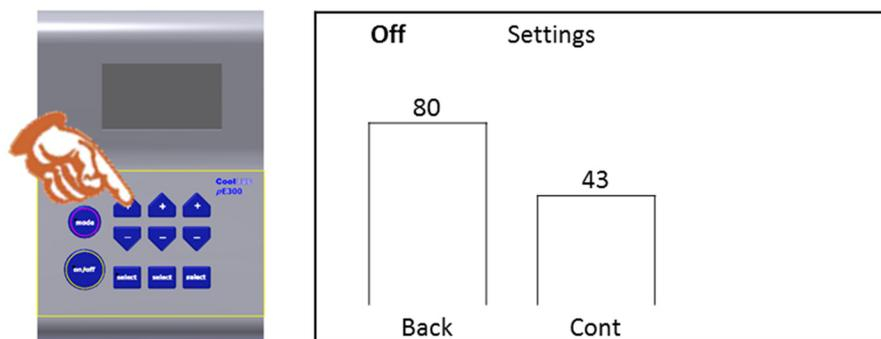
Use the second column up/down buttons to adjust the display contrast as required.
