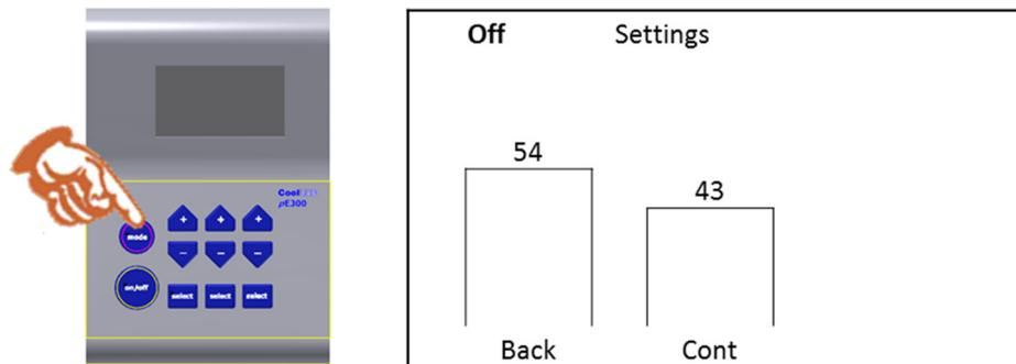
Use the first column up/down buttons to adjust the backlight to the desired level.
