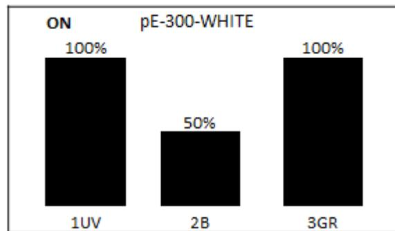
6.7 Individual bands can be switched off (de-selected) by pressing the 'select' button. Light is then only generated where it is required to excite the stains in use. This has many attractive benefits with improvements in contrast, cell viability and savings in energy.
