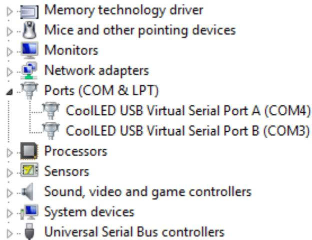
In this example the *pE-300<sup>white</sup>* has been assigned two COM ports, COM3 and COM4. You may need this information to connect to the light source from your software control package. Either COM port may be used for control. Two COM ports have been assigned to allow for diagnostics to take place in parallel with communication and also allow for dual communication should that ever be desired.
